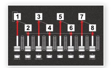
Only faders 2, 4, 6 and 8 are controlling carriers (oscillators). The odd faders are controlling the operators modulating the carriers like 1 modulates 2, 3 modulates 4 and so on. Please take a look at the image and refer to further common FM knowledge materials if necessary. Please also refer to the Performance List 1 which contains informations about used Algorithms.
