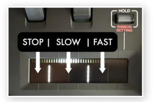
Some Performances are stored with the speed set to "Fast" or "Stop". In this case the Modulation wheels behaves differently. Also the Ribbon Control is not working initially because the Super Knob setting overwrites the value of other controllers. Alternative preferences can easily be changed accordingly and stored if necessary.
